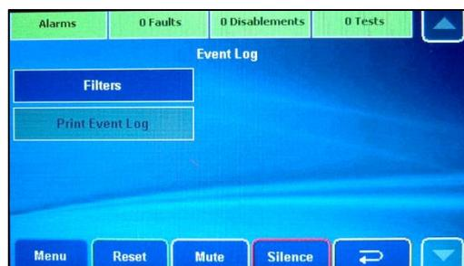
To either filter, or print, the log press one of the blue event log buttons and the window shown left is displayed:
