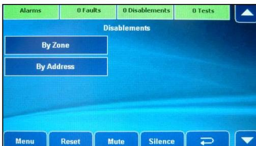
Press the **By Zone** button to select and disable all devices within a specific zone, or press the **By Address** button to select and disable individual devices by entering their loop number and address.
