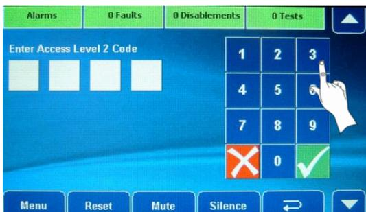
Enter the access level 2 code by pressing the buttons on the touchscreen’s numeric keypad.
